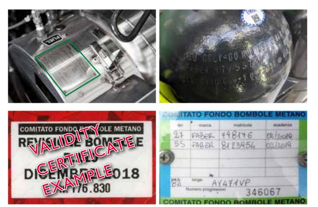
Presence of an up-to-date validity certificate legible for LNG tank and CNG cylinder.
