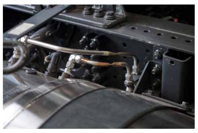
• Rust, dents, breakages and/or gouges  $\rightarrow$  charge for replacement of rigid lines.
