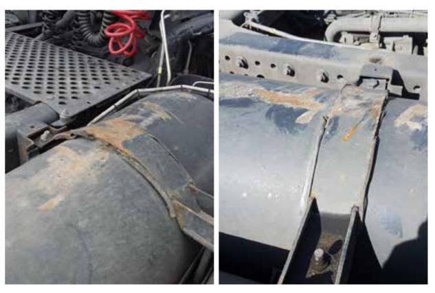
• Rust, dents, breakages and/or gouges  $\rightarrow$  charge for replacement of brackets and bands.
