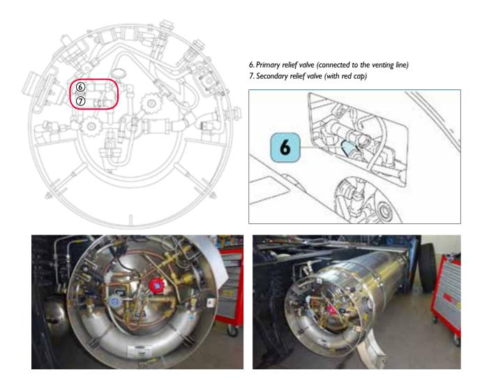
**Important note:** The maintenance plan calls for the mandatory replacement of the primary and secondary relief valves of any LNG tank by the fifth year after manufacture; in case the vehicle is returned after 5 years or more from the contract start date, the customer must ensure that the primary and secondary relief valves has been replaced before returning the vehicle to IVECO.
