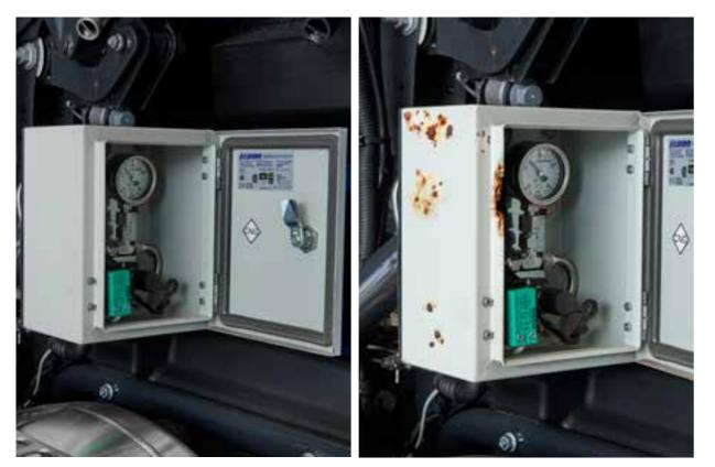
• Rust on the fill receptacle protection box  $\rightarrow$  note without charge for damage.
